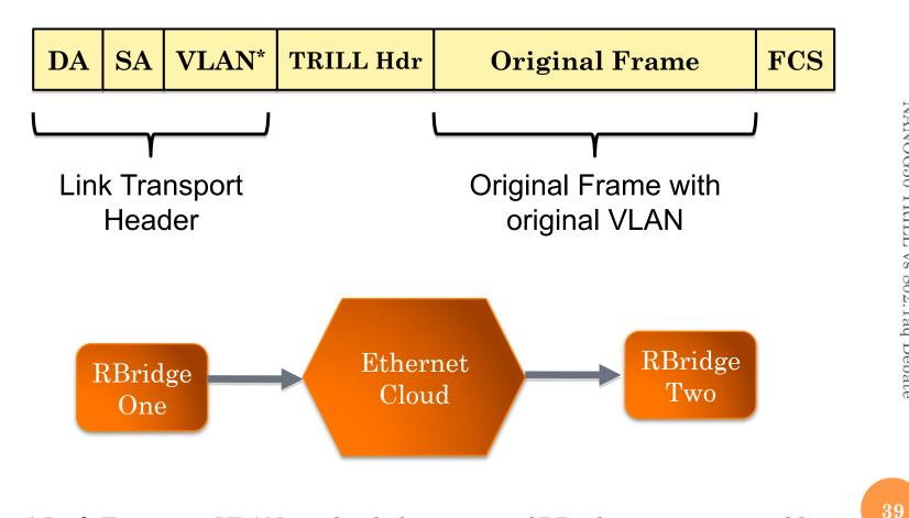
\* Link Transport VLAN need only be present if RBridges are connected by a bridged LAN or carrier Ethernet requiring a VLAN tag or the like.
